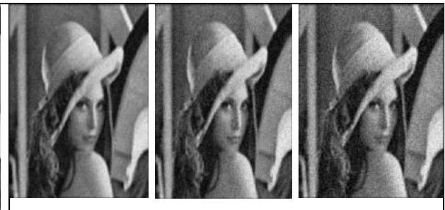
Figure 2: (a-c) Represented blur and noisy images with different level of Gaussian noise ( \sigma^2 = 0.002,0.004,0.006, ) respectively)
