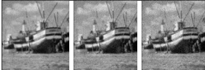
Figure 3: (a-c) represented blur and noisy images with different level of Gaussian noise ( \sigma^2 = 0.002,0.004,0.006, ) respectively);
